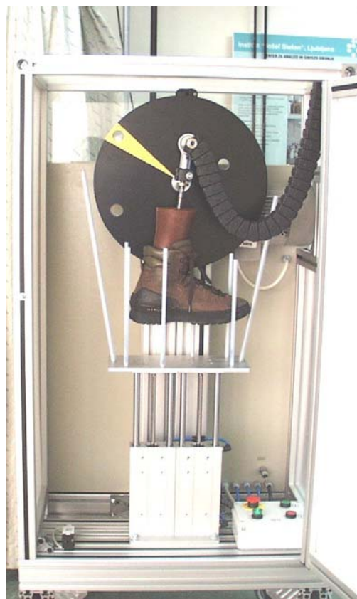
Figure 3: Simulation of gait is achieved by the combined action of the flywheel and pneumatically driven platform (see text for details).
