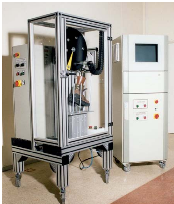
Figure 1: The thermal foot manikin system comprises three components: the Gait Simulator (left), the heated Thermal Foot Manikin (attached to the flywheel of the gait simulator), and the Control Unit (right).
